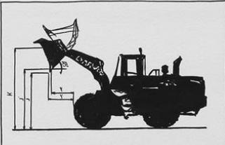
2. The machine itself is articulated centrally beneath the operators cab allowing the machine a certain amount of flexibility both in the central axis (see top image) but also between the axles of the machine. The range of the bucket means that it can only dig (excavate) on a level surface and is generally seen in gravel or sand quarries where its large capacity front bucket can be used to load trucks from the side.
