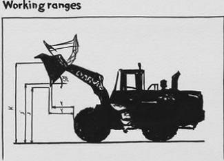
2. The machine itself is articulated centrally beneath the operators cab allowing the machine a certain amount of flexibility both in the central axis (see top image) but also between the axles of the machine. The range of the bucket means that it can only dig (excavate) on a level surface and is generally seen in gravel or sand quarries where its large capacity front bucket can be used to load trucks from the side.
